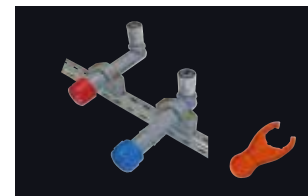
BUTE-1 Adjustable 1/2" BSP Male Wall Elbow BUTE1 - 1/2" BSP x 15mm x 70mm BUTE1EX - 1/2" BSP x 15mm x 100mm Includes telescopic steel brackets, test caps (hot & cold) and palm spanner.
